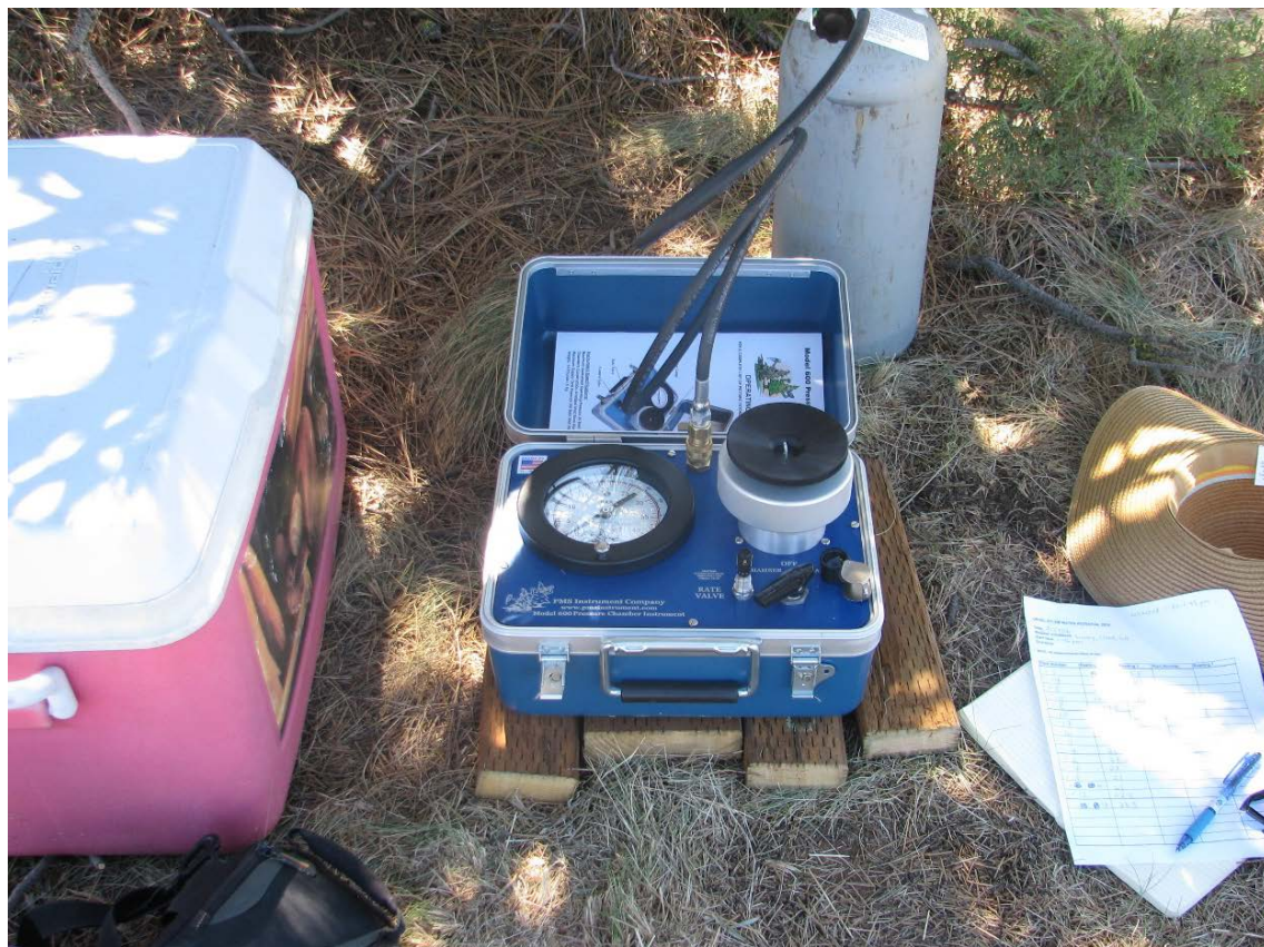
Figure 4. Using a Scholander-type pressure chamber to measure xylem pressure potential.
